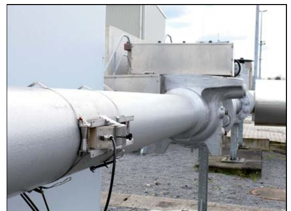
Measurement with explosion proof transducers
